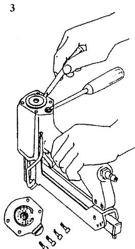
punch of 3,5 mm. Replace damaged parts and grease piston O-ring 13300131 before refitting with special grease 13301706
