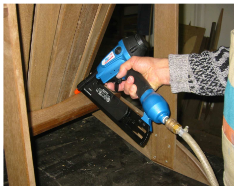
26° magazine: Narrow working places always visible, even in corners and angles.
