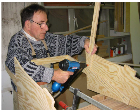
26° magazine: Exact placement of brads. No marks on sensitive surfaces.
